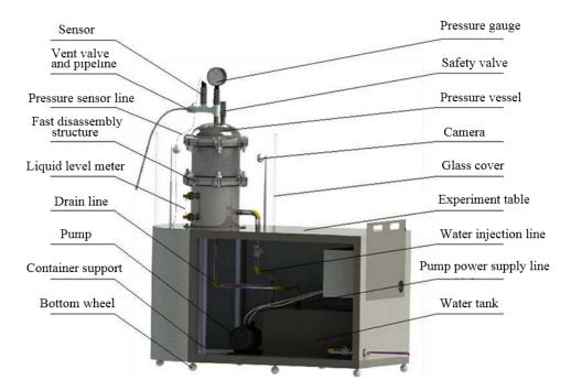
Figure 2: Experimental station whole structure design and piping layout.
