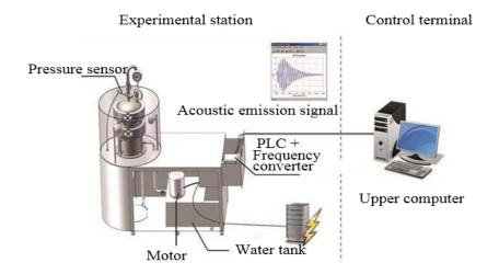
Figure 3: The overall design of the remote control on-line NDT experimental station.
